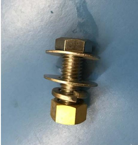
This is the bolt and washers to be used to connect the paddle to the switch on the under arm change event.
